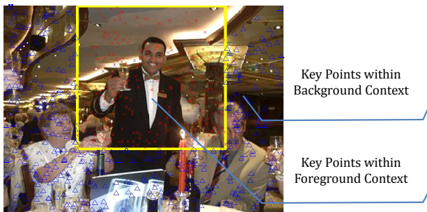
Figure 4. An illustration of the context feature extraction process. The yellow rectangle denote the division of the defined foreground and background context areas. The blue triangles and red crosses denote the SIFT key points belonging to background and foreground respectively. For better viewing, please see original color pdf file.
